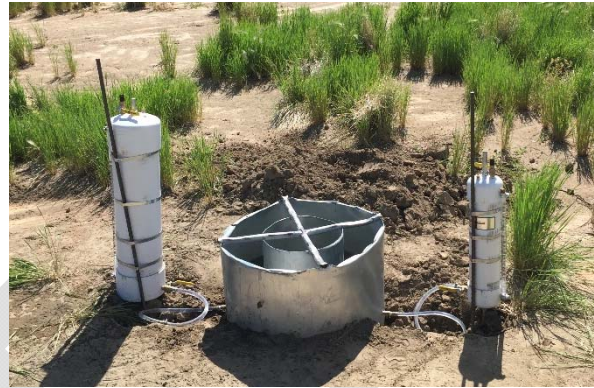
Photograph 1 - Double ring infiltrometer test in Rapid Infiltration Basin 10.
