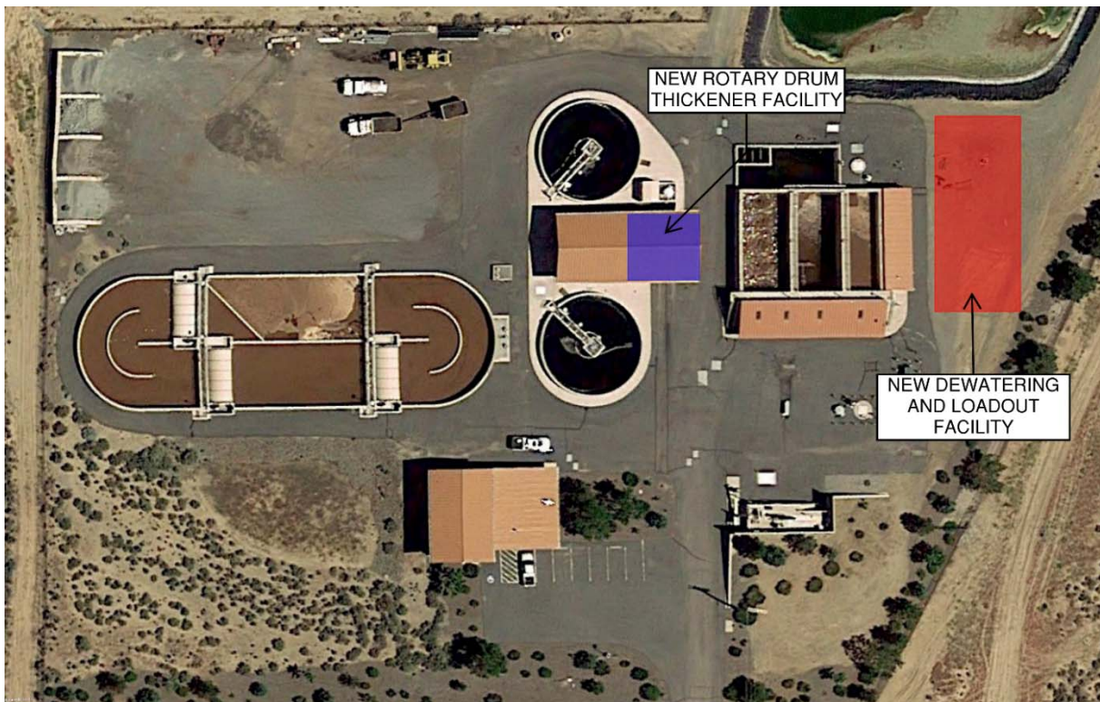
Figure 5-11: Option 1 Digestion and Dewatering Improvements
